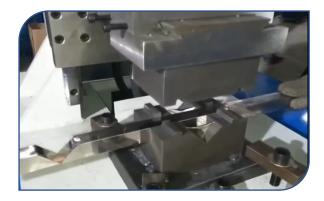
The machine can bend pipes of different sizes by changing the molds
