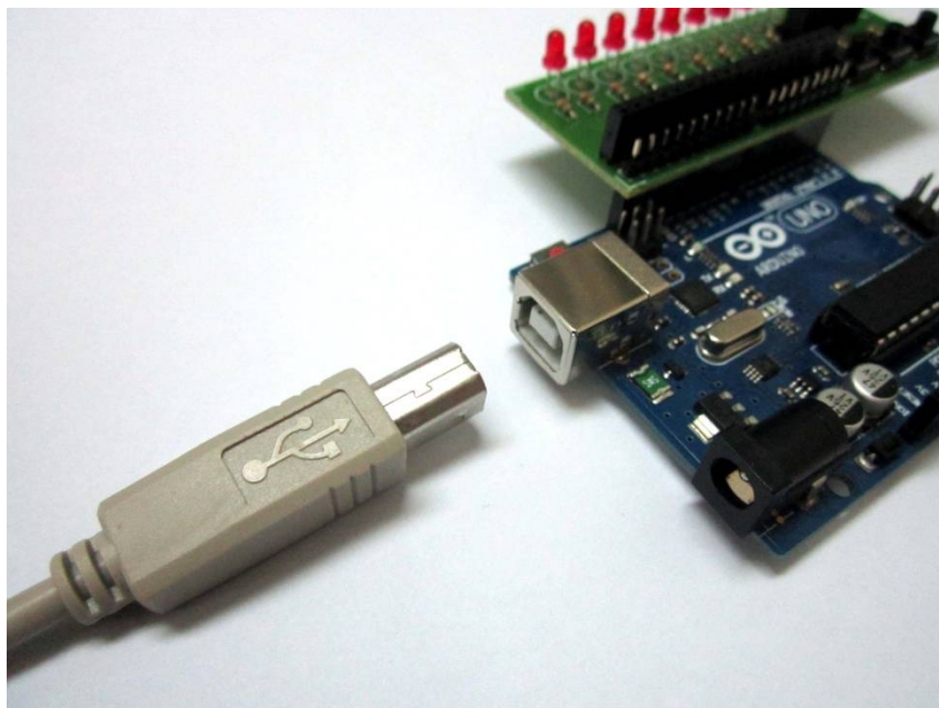
Figure 10. Wiring the USB cable
