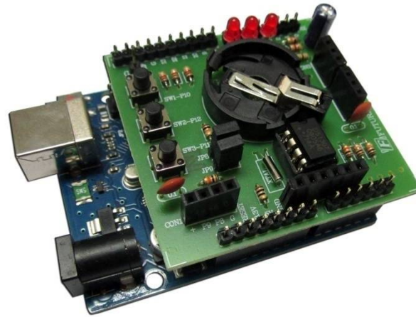
Figure 9. Connecting FK1417 board with Arduino UNO R3 board
