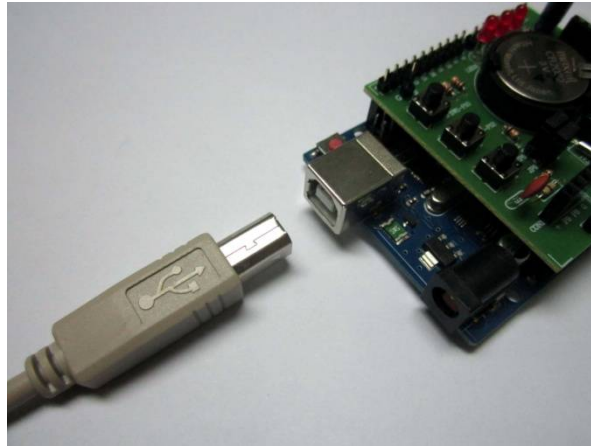
Figure 11. Wiring the USB cable
