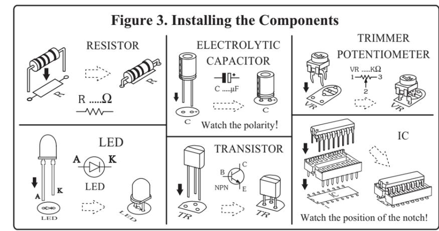
Figure 3. Installing the Components
