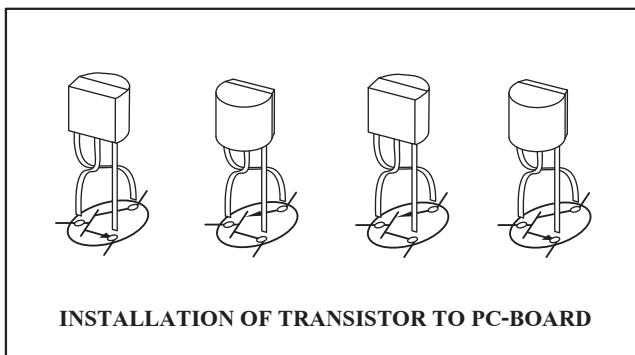
INSTALLATION OF TRANSISTOR TO PC-BOARD
