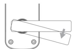
Press down the inside handle to open while locked.
