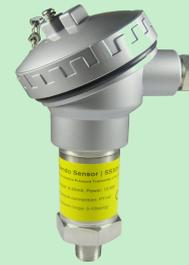
SS302 series adopt a high performance piezoresistive pressure transducer as the sensing part, the inner structure is O-ring sealed,  $-10$  to  $70^{\circ}\text{C}$  wide temperature compensation, well suitable for precision applications in industrial environments for pressures ranging from 0,1 to 1000 bar, liquids or gas.
